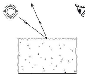
If you look at the two diagrams illustrating a shiny finish and a smooth finish, it can be observed that the shiny surface is shown as a perfectly straight line while the opaque surface is shown as an irregular line.
